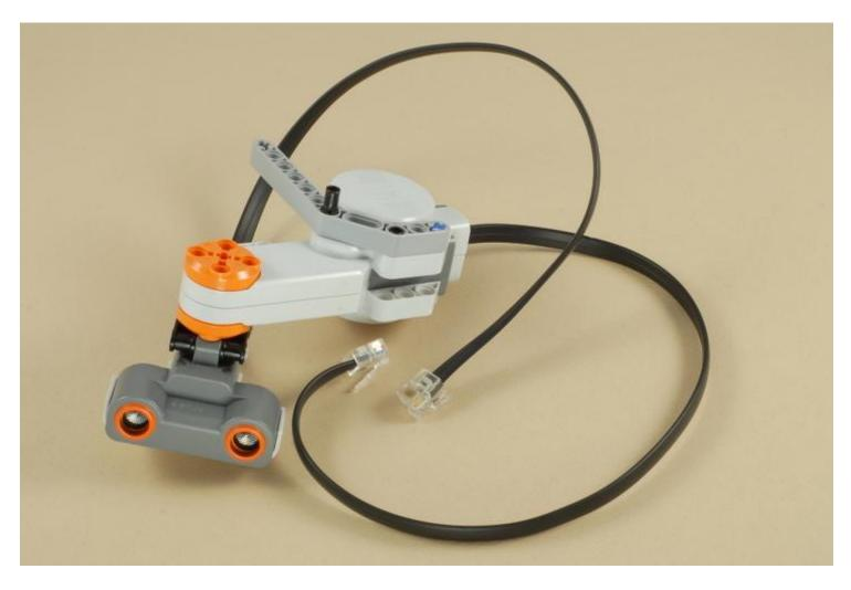
Connect the neck motor wire to port A on the NXT, and the ultrasonic sensor wire to port 4 on the NXT.
